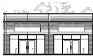
HORIZONTAL METAL PLANKS ECHOING THE FEEL OF WEATHER BOARDING
