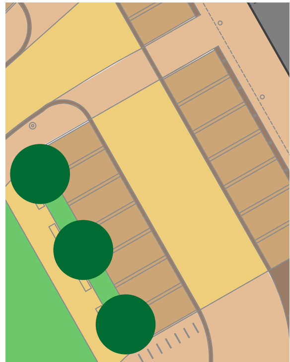
BACK EDGE OF PARKING BAYS 3 ROWS OF TEGULAR SETTS WITH BOLLARDS AT 2.4M CENTRES
