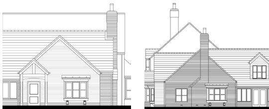
PUB ELEVATIONS (BELOW) DESIGNED TO HAVE A KENT CHARACTER WITH WEATHERBOARDING, RED BRICK, TILED ROOF, GLAZING BAR PATTERN AS SHOWN IN THE EXAMPLES ABOVE
